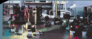
The picture shows part of Zewail's "camera". It is a complex array of lasers, mirrors, lenses, prisms, molecular beams, detection equipment and more.
